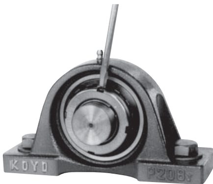
Fig. 14.8 Bending outer tab of washer (Locking locknut)
